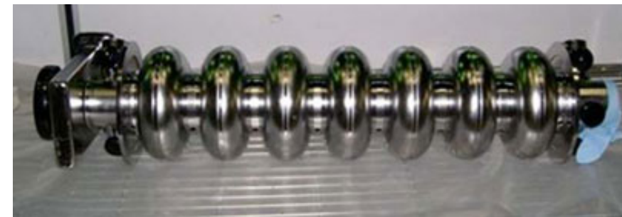
Seven-cell, High-Gradient Niobium SRF cavity for 12 GeV Upgrade
